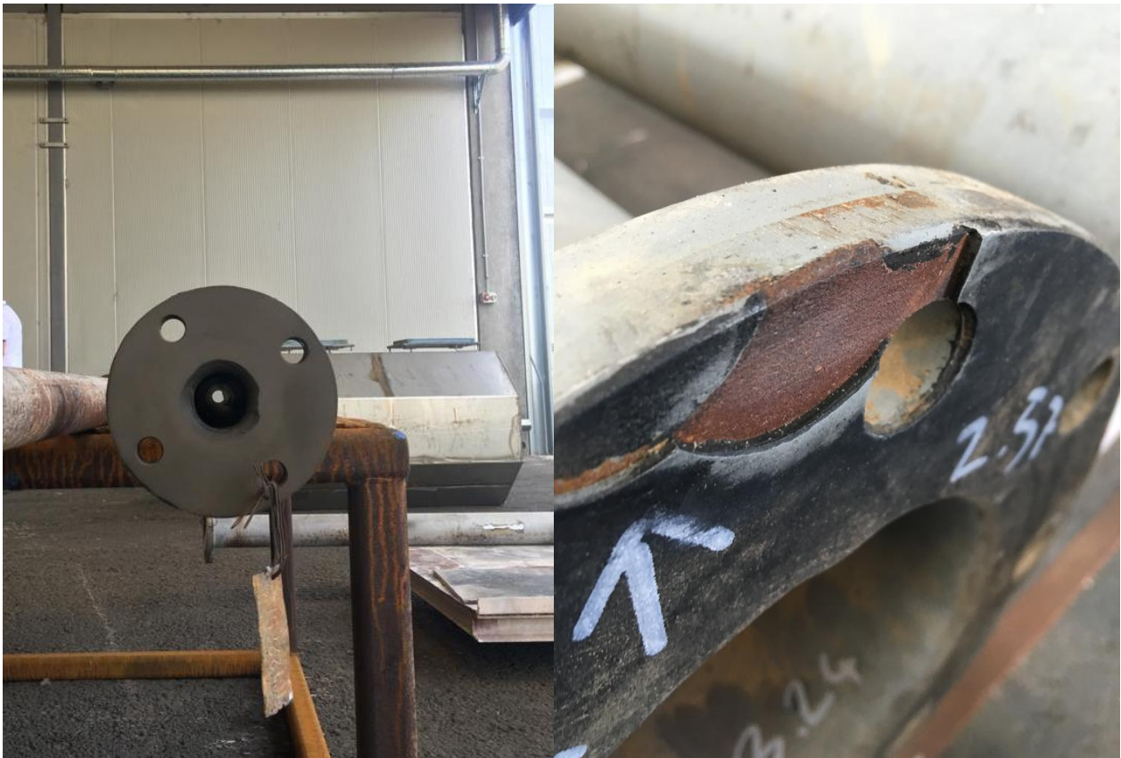
Figure 1.2 Adhesion Problems with Abu Qir's Hard Rubber Pipes
