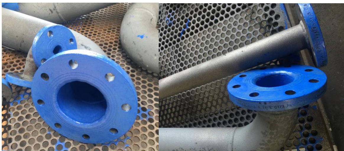
Figure 1.6 New Adhesion on the pipe surface is obtained thanks to the application of a special glue on it
