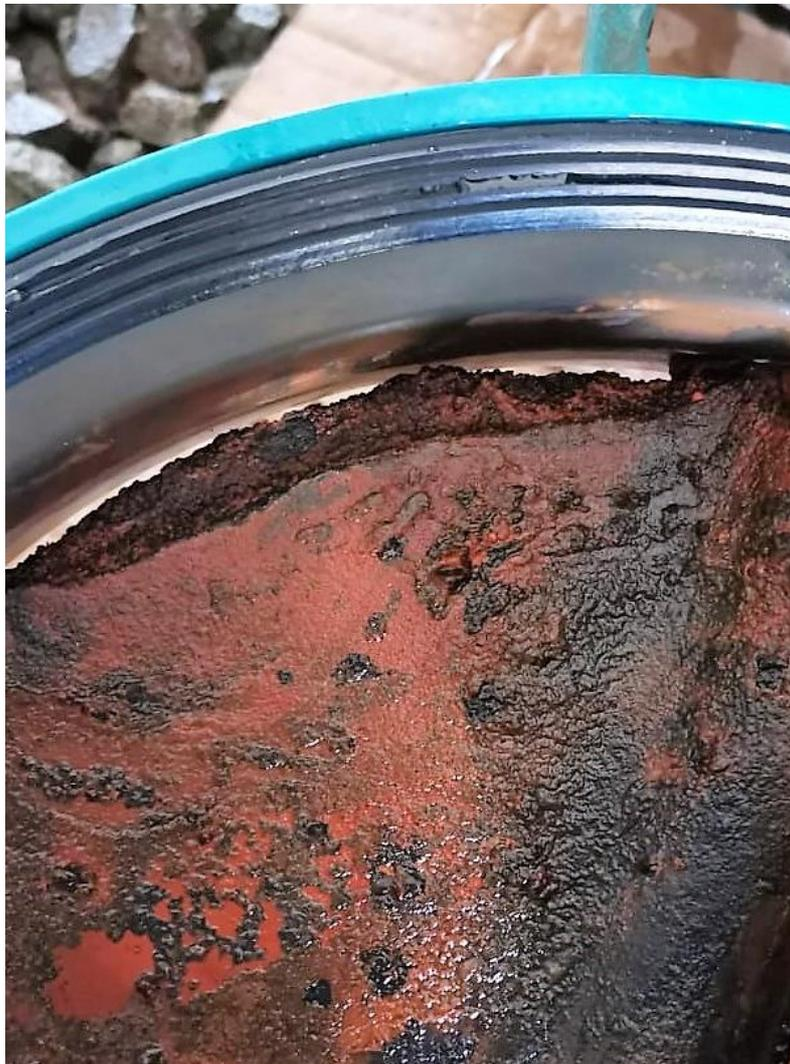
Figure 1.2 High corrosion of a Dhuba SWRO Plant's Butterfly Valve
