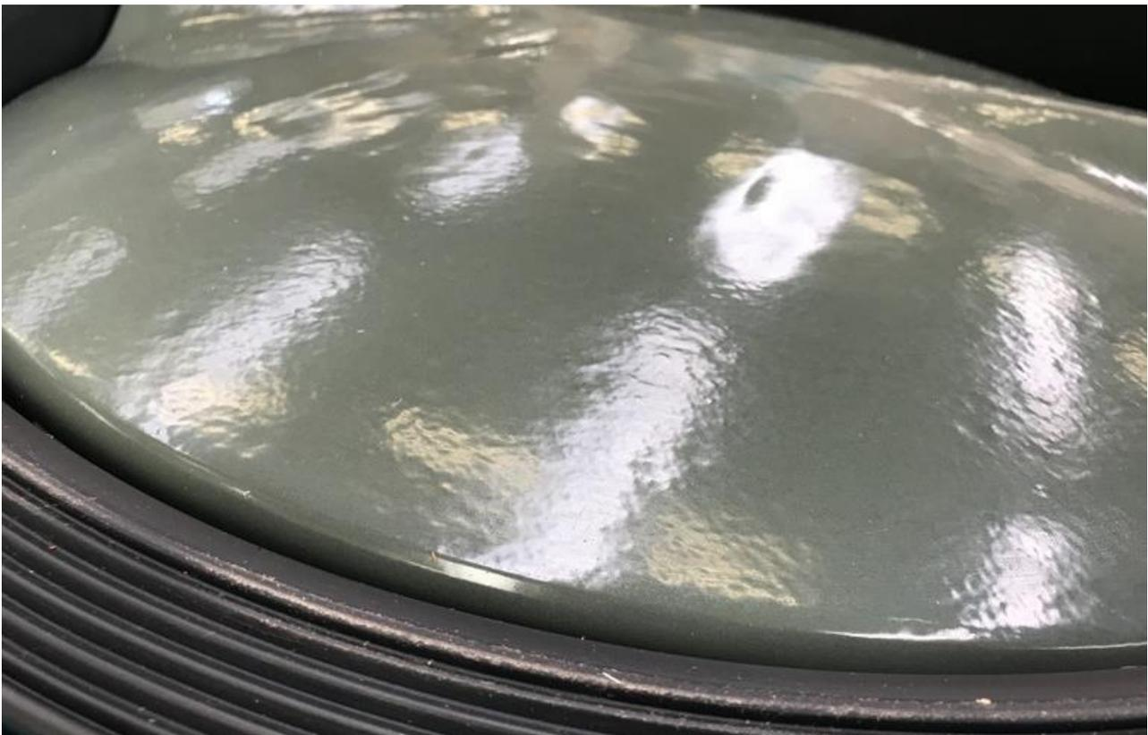
Figure 13 Halar Coated Butterfly Valve Disc
