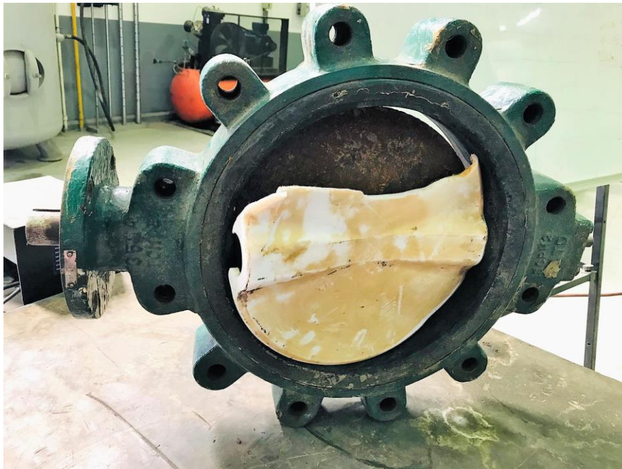
Figure 1.1 Lug type Butterfly valve damaged by the hard environment of a mining application
